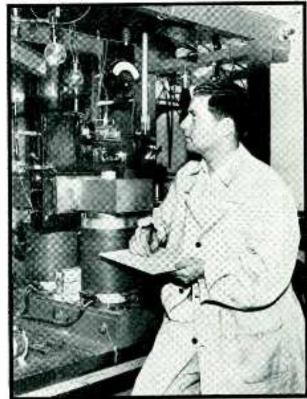
The latest mass spectograph at the University of Chicago will detect differences in weight of the order of 10^{-26} gram. Atoms from a hot spark are drawn through a slit, acted on by magnetic and electric fields, finally hit a photographic plate, forming a spectrum which reveals the relative weight of the atoms
