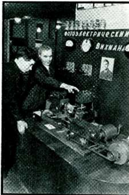
This automatic metal-working lathe shapes its work from a black-and-white pattern which is scanned by a photocell. It was designed by a Russian, V. S. Vikhman
